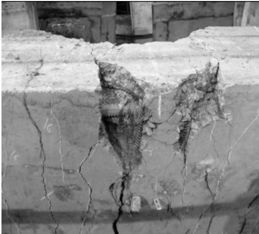
Figure 6 – Destruction of the model under the action of the ultimate load
