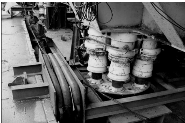
Figure 2 – Pneumatic and pneumohydraulic devices for the formation of the required frequency composition of seismic action
